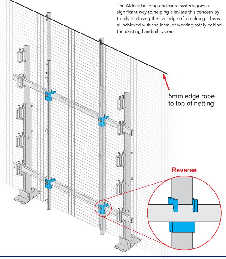
THIS IS A DEBRIS RESTRAINT SYSTEM ONLY. THIS SYSTEM SHOULD ONLY TO BE USED IN CONJUNCTION WITH THE ALDECK TELESCOPIC HANDRAIL SYSTEM.
